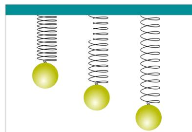
$$1. \ a) \ T = 2\pi \cdot \sqrt{\frac{m}{D}} = 2\pi \cdot \sqrt{\frac{0,10\text{kg}}{20\text{N/m}}} = 0,444\text{s}$$
